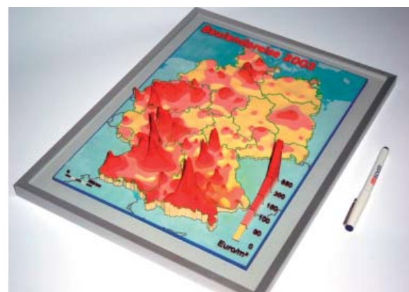
Figure 8: Physical 3D model produced by 3D printing, representing a smooth surface interpolated from polygon-based data.
