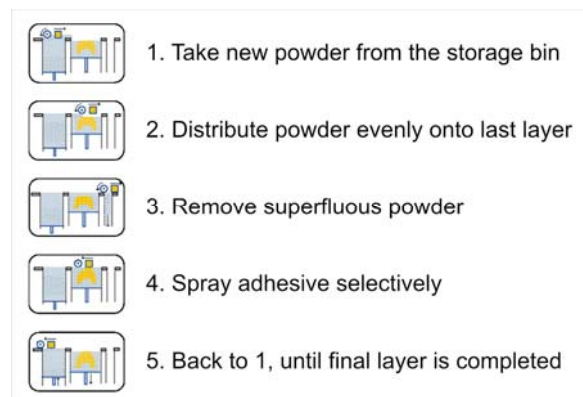
Figure 1. Building steps for 3D printer Z510
